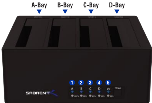
1.A-Bay LED / 2.B-Bay LED / 3.C-Bay LED / 4.D-Bay LED / 5.Power LED
